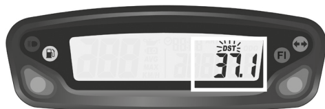
Fig 6 Adjustable trip distance function
