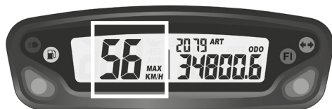
Fig 2 MAX speed function
